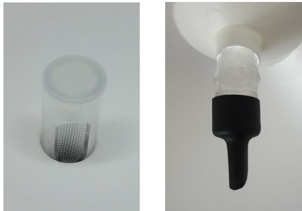
Figure 4 - Filter and filter cap (left) / Nozzle delivering water into tipping bucket (right)
