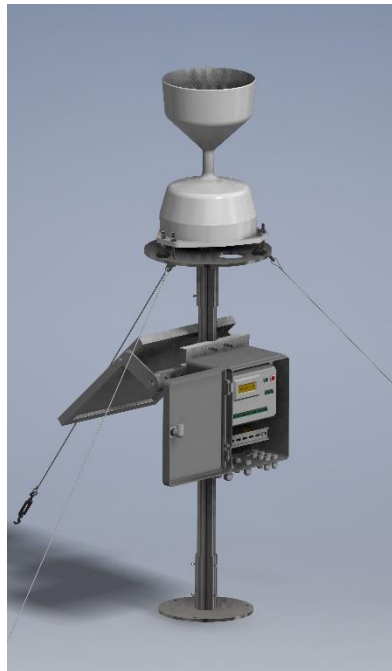
Figure 3 – Rain gauge fitted to a pedestal as part of the EML system
