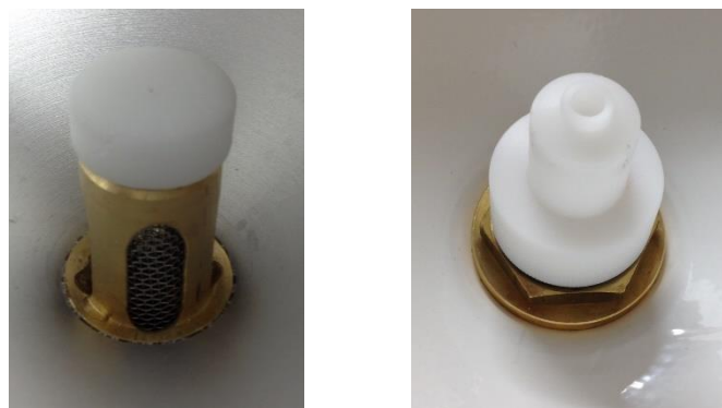
Figure 4 - Filter and filter cap (left) / Nozzle delivering water into tipping bucket (right)
