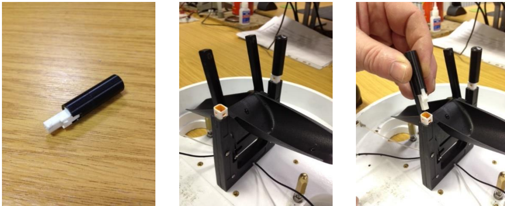
Figure 6 - SBS replaceable reed switch (0.2mm version) (left) / Empty socket to house one of the reed switches (centre) / reed switch being inserted into the empty socket.
