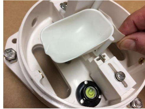
Figure 7 - Removal of bucket
