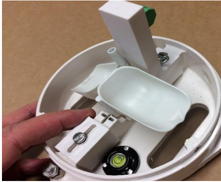
Figure 6 - Pivot holding piece
