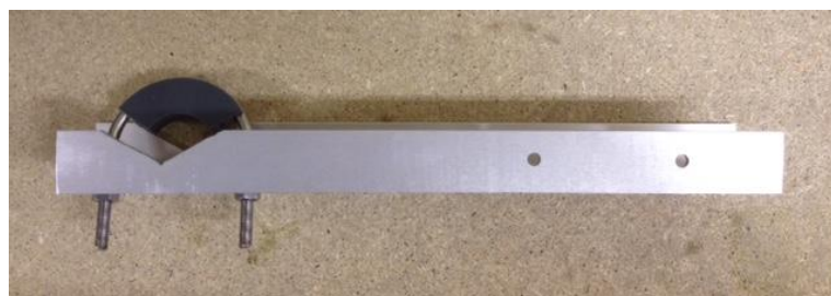
Figure 12 - Aluminium mast mounting arm
